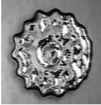
FIGURE 2. View of a defect in the azimuthal pattern owing to the contact between the liquid metal pool and the substrate (the initial drop radius is a = 30 mm, f = 8.050 Hz, I = 140 A).
